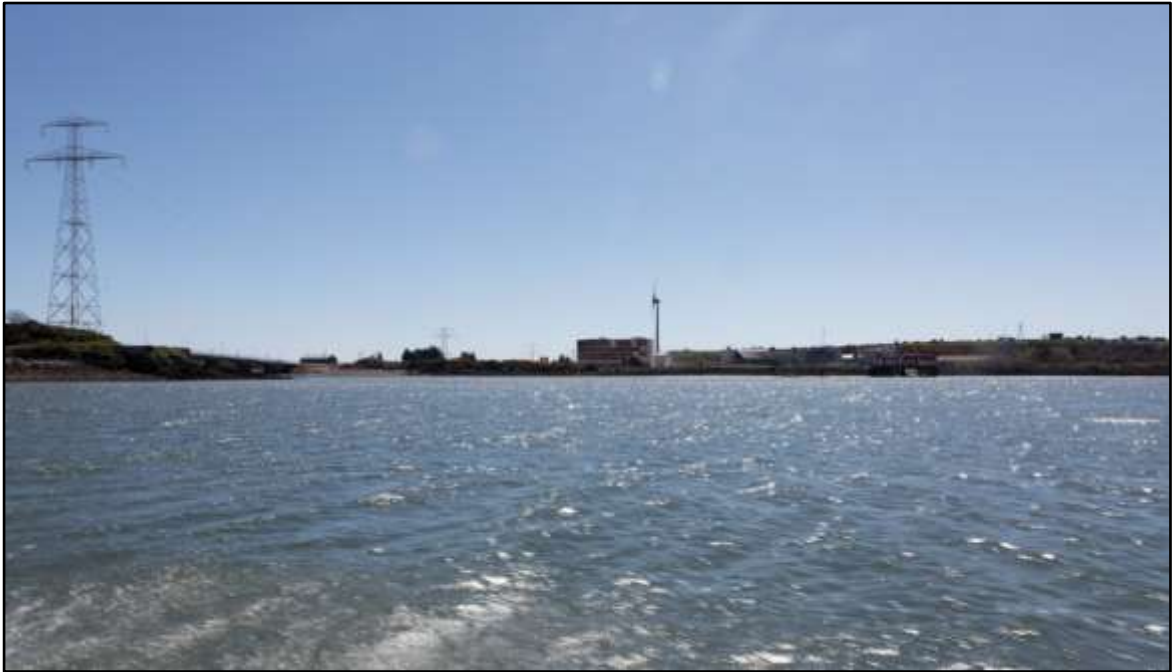
Figure 9 – the climb out from the Main Square as viewed from ground level on the shoreline of Haulbowline. (Note that as the aircraft lifts to the hover and then proceeds to climb away the perspective of pylons and other obstructions will alter as they “descend” below the skyline making them and the power cables much more difficult to see; this will not be the case with the turbine).
