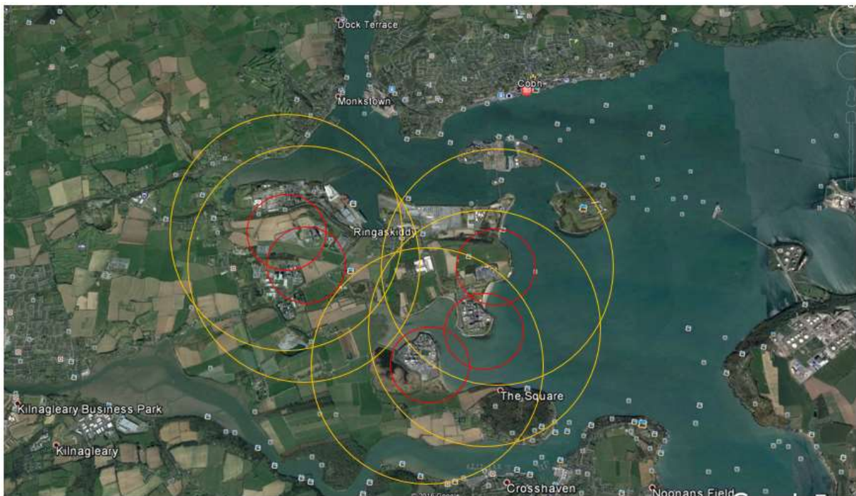
Figure 11- turbulence areas behind the operating and permitted wind turbines (depending on wind direction).
