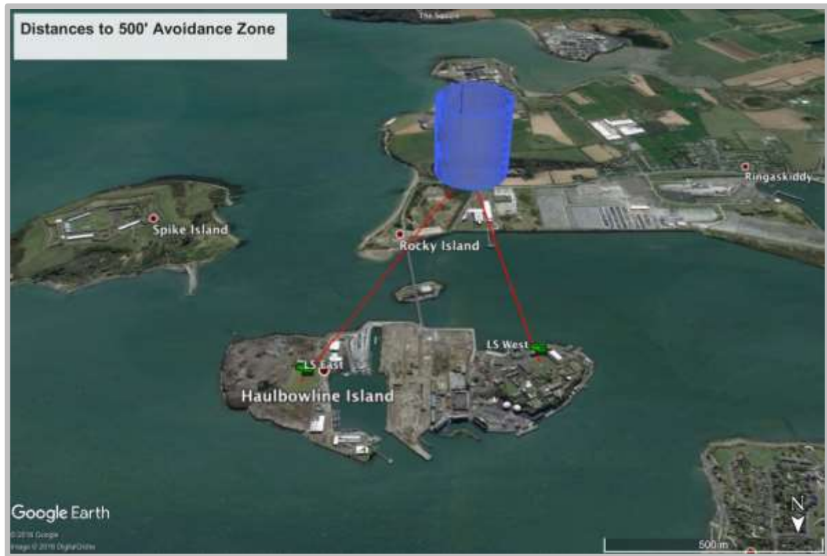
Figure 15 - Distances to the stack avoidance zone from the HNB landing sites
